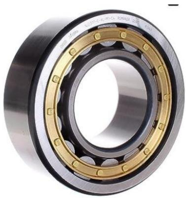
Product details NU230E.M1.C3 Cylindrical Roller Bearing, Removable Inner Ring, 150mm Bore Dia., 270mm Outside Dia., 45mm Width, Brass Cage Manufacturer?:?FAG
