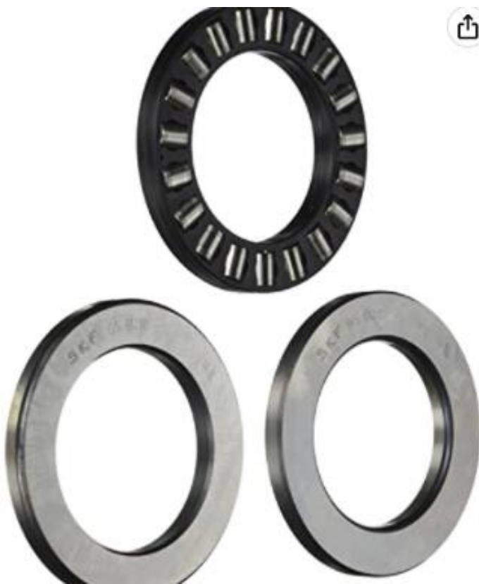
SKF 81214 TN Cylindrical Roller Thrust Bearing, Polyamide/Nylon Cage, Metric, 75mm Bore, 110mm OD, 27mm Width
