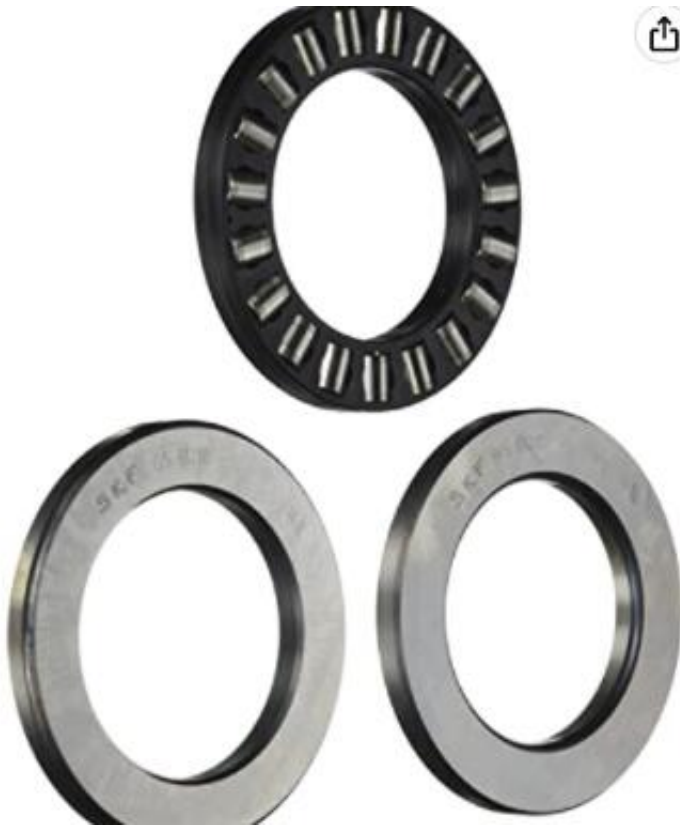
SKF 81120 TN Cylindrical Roller Thrust Bearing, Polyamide/Nylon Cage, Metric, 100mm Bore, 135mm OD, 25mm Width
