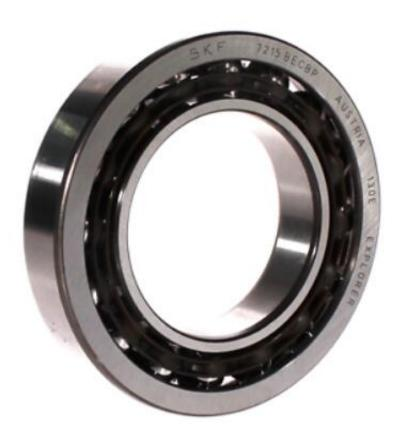
The 7215BECBP SKF is a single row angular contact bearing. These bearings have solid inner- and outer rings. They owe their name to the contact angle that is created as the raceways of the inner and outer rings are offset from each other along the bearing axis
